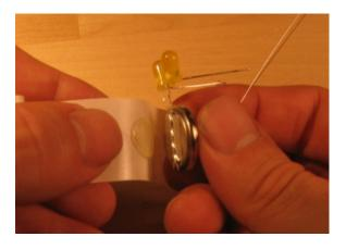
Firmly press against the backing, so that the glue dot adheres to the bottom of the battery, like so:
