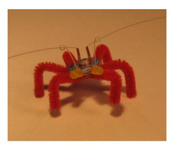
When an antenna is moved slightly, it contacts the loop and turns that eye "on:"
