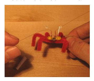
Slip each tube over each looped antenna lead:
