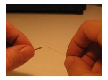
Slide the tube about  $\frac{1}{2}$  of the way down the length of the wire. Use the ruler to help center it; there should be 5  $\frac{3}{4}$ " of wire extending from either end of the tube. You use a little piece of tape to help keep the wire in place, like so:
