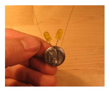
IMPORTANT: Make sure the foil does not touch the side of the battery! It shouldn't get any closer than this:
