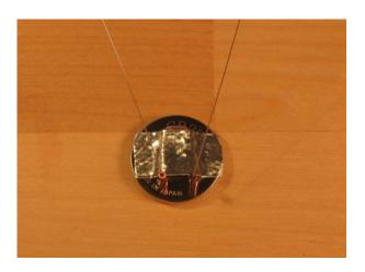
Put the antennae / battery assembly aside for now. Next, grab the remaining, smaller piece of foil tape, and peel off the backing. Pick up the LED eyes, holing on to them by one of the looped leads, and hold it upside down. Position the foil against the *twisted* LED leads, like so:
