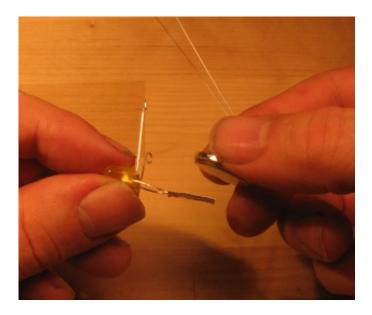
Now firmly press the tape against the bottom of the battery, working it in to all the nooks and crannies so that it will stick well:
