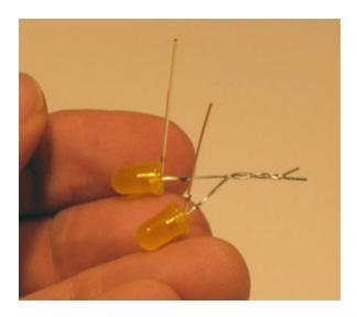
You may notice a bit of "jiggle." This is easily remedied by giving the twisted leads a good squeeze with the pliers, like so:
