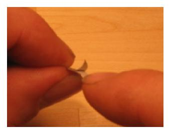
Try not to touch the sticky side, or it won't stick as well. (This foil has a special adhesive that conducts electricity, to help your Blinkybug light up).
