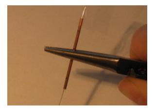
Next, using your thumb while firmly holding the copper tube in place with the pliers, bend each end of the copper tube 90°:
