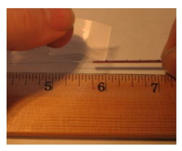
Now, with your needle-nose pliers, grab the copper tube right between the two center-most marks (those at 5/8" and 7/8"); you should have equal amounts of copper tube and wire extending from either side of the pliers:
