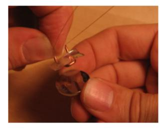
Now press the foil tape so that it sticks to the surface of the battery:
