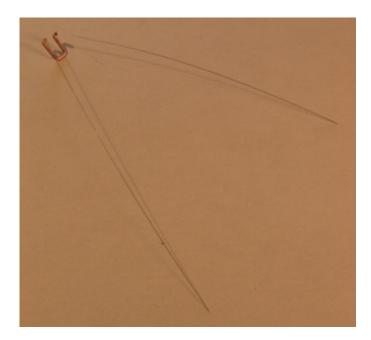
Next, you want to add little flaps to the ends of the antennae; this will make it far more sensitive to light breezes. Tear off a 1 ½" strip of cellophane tape, and stick it on the end of one of the antennae so that the end of the wire extends about half-way down the length of the tape:
