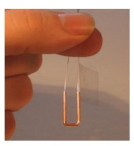
If one section of copper tube is slightly longer than the other, don't worry about it... this is not an exact science! You can now remove the bit of tape. Here is another view of what we have so far (don't worry if the wires cross like this or not):
