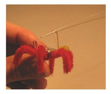
To get everything lined up just right, you will probably need to make some adjustments. If an antenna wire is way off, you can gently crimp it where it comes out of the copper tube, as you did earlier (the antenna may need to come out of the loop to do this):
