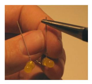
Now give it a twist in the *outward* direction, making a small loop:
