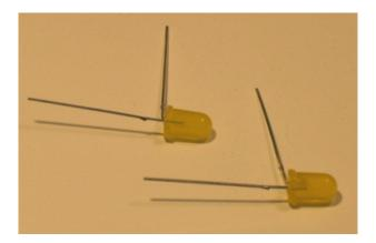
Next, you want to twist the 2 shorter (negative) leads of the LEDs together. First, with the LEDs pointing in the same direction, and the positive leads parallel to each other, cross the ends of the two negative leads, like so:
