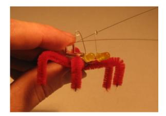
For more fine adjustments, hold the body of the bug while gently positioning the loop by grabbing the LED lens or the lead itself:
