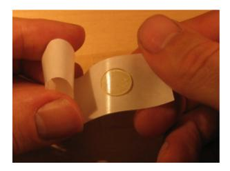
Try not to touch the dot itself (this will decrease its stickiness). Place the exposed dot against the bottom of the bug assembly, against the negative side of the battery, and directly over the twisted LED leads:
