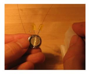
Now pick up the leg assembly, which will be attached to the bottom of the battery:
