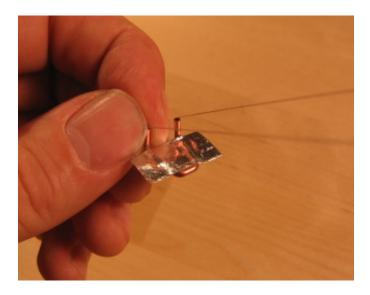
There should be about 1/4" of extra foil extending from either side of the copper tube.
