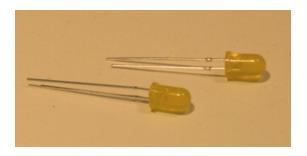
Notice that each LED has 2 wire leads, and that one lead is slightly longer than the other. The long lead is the "positive" lead... this is important, as LEDs need to be oriented the right way, or they don't work!
