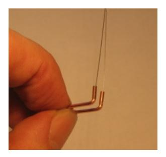
Next you need to bend the music wire where it exits the tube so that it sweeps forward—that is, in the same direction as the bent copper tube. Because this wire is "springy," you need to really mash it a bit with your finger. Push down firmly on the wire as shown here:
