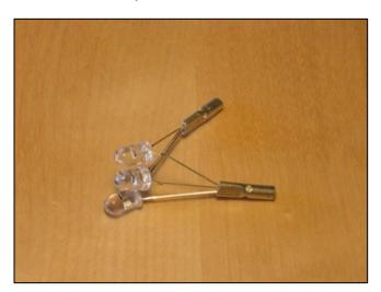
4. Wire LEDS to the Battery Case Take the end of the red wire lead from the case and insert it into the open end of the butt splice that is attached to your *positive* LED leads:
